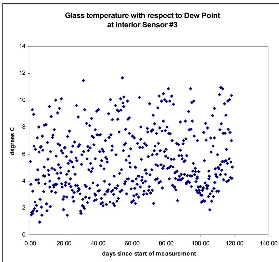
**Figure 13: Estimated glass surface temperature with respect to the Dew Point of the interior air near the centre of the central lancet**
