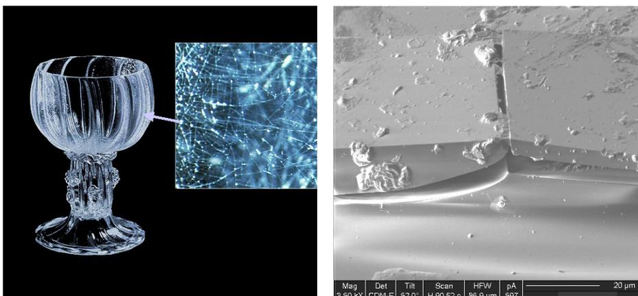
**Figure 11: A Ravenscroft goblet exhibiting a network of surface cracks, and a micrograph of glass which has started spalling after exposure to water vapour (illustrations courtesy of Sarah Fearn)**
