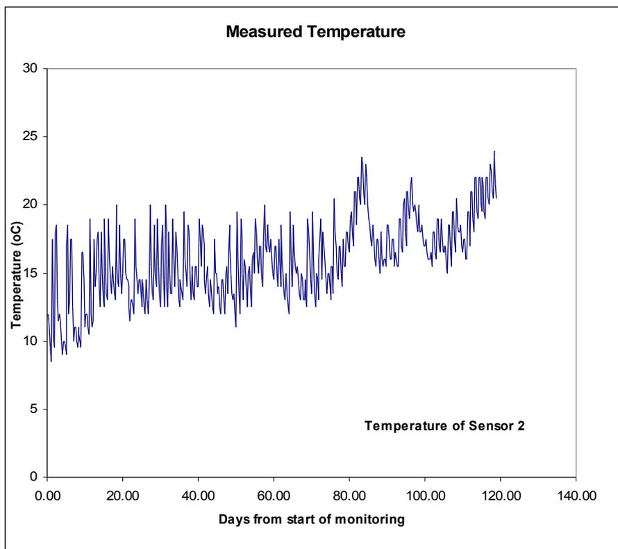
**Figure 4: Interior air temperatures measured mid way up the left hand lancet window**
