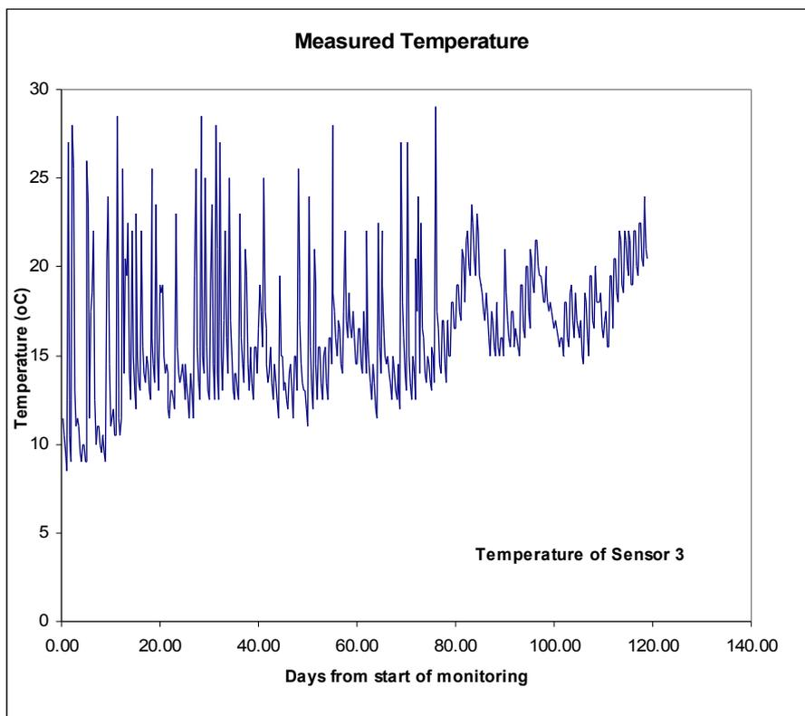
**Figure 6: Interior air temperatures measured mid way up the central lancet window**
