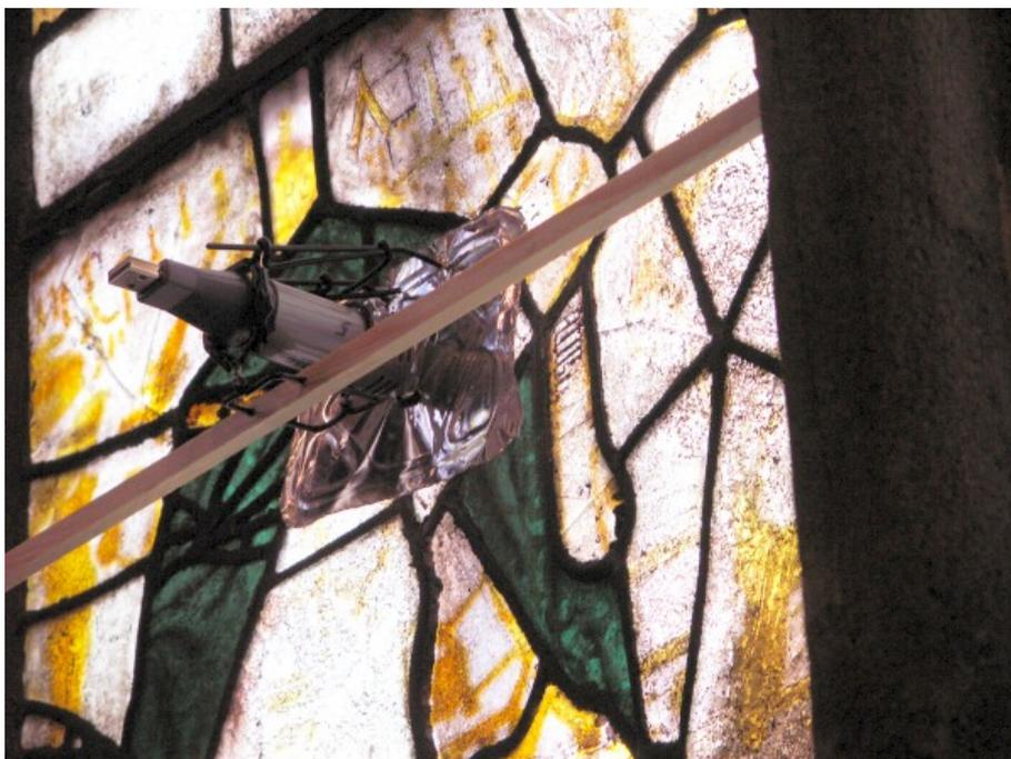
**Figure 1: Air temperature and humidity sensor mounted within the lancet**
