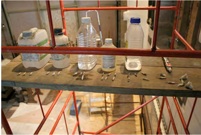
Context view of cleaning trials in progress when the range of solvents/materials known to work on the different materials present are trialled and then evaluated to determine the safest most effective technique/material.
